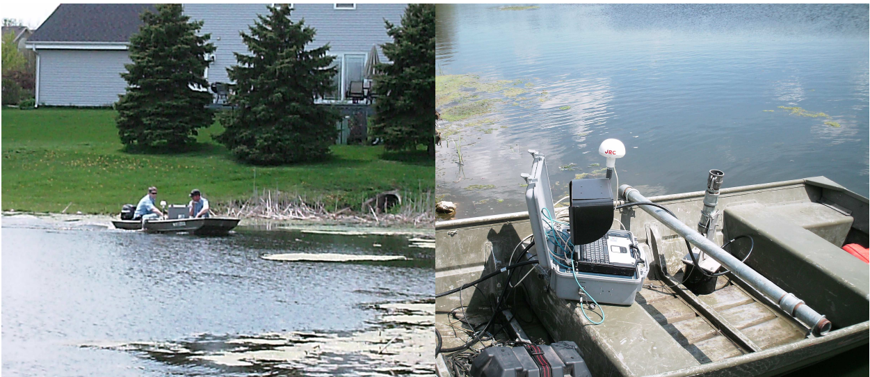
Photo showing Hydro Acoustic data collection and lake level (left) and photo of digital Hydro Acoustic mapping equipment
